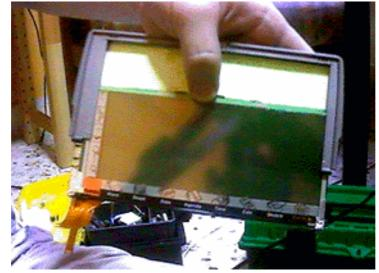
Now slide the screen back into the casing ensuring the corrugated plastic sheet stays in place.
