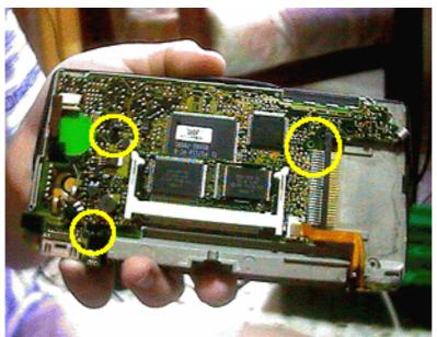
Close the lid slowly to pull the flexi's through the slot and seat the motherboard in the chassis. Insert the three screws and tighten GENTLY!
