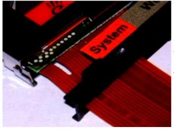
reassembly is essentially the reverse of opening. Feed the flexi and protector through and clip the icon labels back onto the screen.
