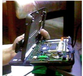
Clip the battery compartment onto the back. Flip the Psion over and clip the front edge of the bottom cover in then hinge down over the back. Tighten the three screws to secure it.
