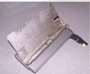
Fold the screen right back and clip the springs into the outer hooks. Then flip the screen back to normal position and insert the flexi through the chassis slot. Clip the springs back under the lugs in the center of the battery compartment
