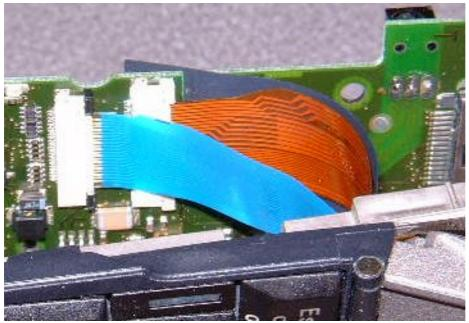
Insert both flexi's into the main board sockets ensuring the black or brown protector end fits through the narrow slot in the main board. The screen flexi should be pushed into the socket so that no gold is showing. The end is a very good fit to ensure that the contacts align, if necessary grip the flexi with some small FLAT pliers and push in gently. Then push the two lugs on the connectors away from the flexi's to secure them.
