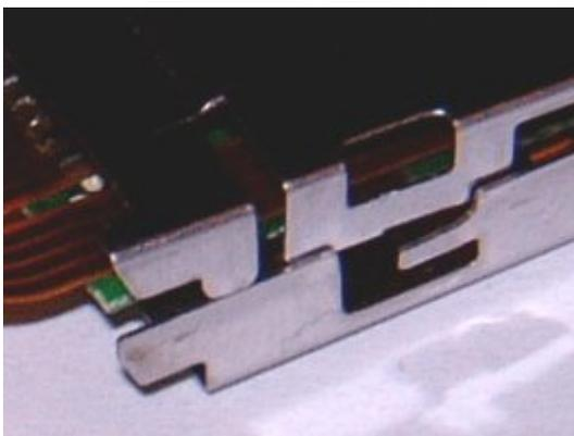
Now attach the metal back of the screen assembly by clipping in the two lugs at the top and 'hinging' the back down. Ensure the sides of the back go INSIDE the front metal cover. Push the small prongs back into the holes ensuring that nothing is proud of the outer case or the screen assembly will not fit back into the casing.
