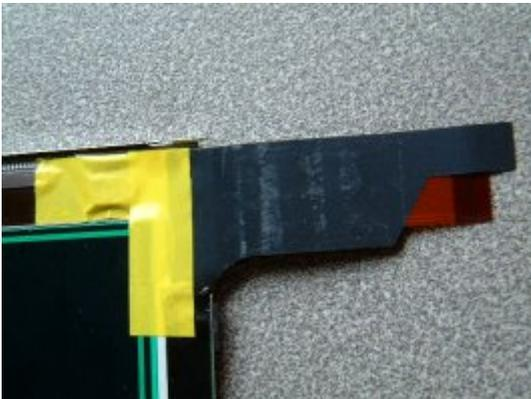
Tape down the touch screen flexi using pressure sensitive tape. Use some more double sided tape across all the exposed main flexi solder joints to stick the black or brown flexi protector back to the screen. Ensure that the protector is aligned with the flexi itself. Add some more pressure sensitive tape over the protector to hold this down.
