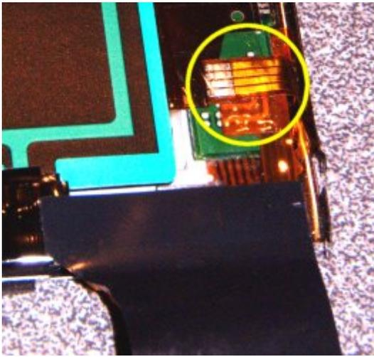
Now stick the remaining 'tail' part of the flexi to the touch screen connections using double sided tape ensuring that the solder connections are aligned. Solder the four touch screen connections to the other part of the flexi. You may find that the two flexi's need holding together with some locking tweezers or similar to stop them springing apart.
