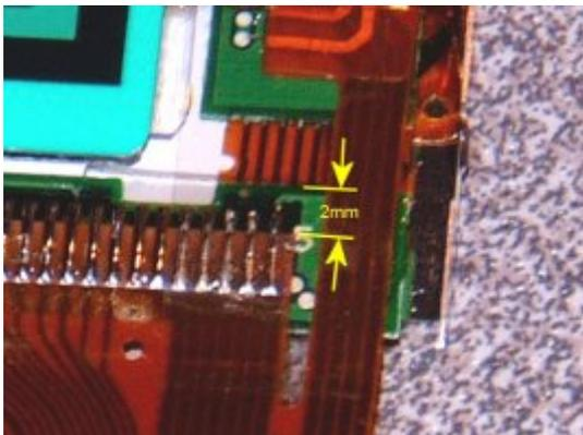
Now carefully align the new flexi with the contacts and stick it down to the double sided tape. The flexi should be approx 2mm from the top of the green PCB. The dimension is not critical but the flexi must be parallel with the screen edge. You can check this by putting a ruler along the metal screen edge.
