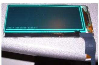
need to remove the back case. Do this by gently bending the small tabs (three each side and four at the bottom) out and then lift the back cover off (bottom first). The picture shows what underneath the green rectangle is the EL backlight and the black/ brown tape is the flexi protector. (The brown version looks just like another flexi, however it
