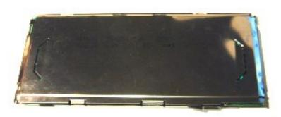
First we must remove the icon labels from the screen assembly. This simply unclips from the three lugs on the front of the screen (no lugs at the back). Use a thumb nail between it and the screen to remove.
